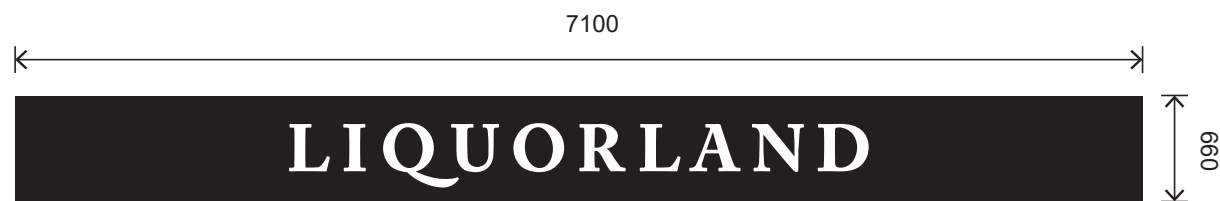
SIGN 3 WALL SIGN / NON - ILLUMINATED 2mm Aluminium panel, digitally printed, with all edges to be wrapped. QTY. 1 Size: 7100mmW x 660mmH
