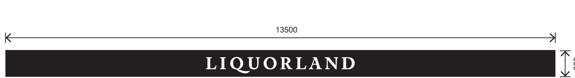
SIGN 2 FRONT CANOPY SIGN / NON - ILLUMINATED 2mm Aluminium panel, digitally printed, with all edges to be wrapped. QTY. 1 Size: 13500mmW x 660mmH
