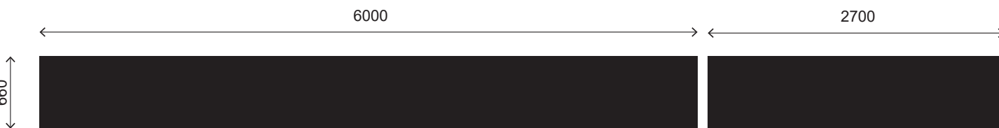
SIGN 8 CANOPY SIGN / NON - ILLUMINATED 2mm Aluminium panel, digitally printed, with all edges to be wrapped. QTY. 1 Size: 6000mmW x 660mmH 2700mmW x 660mmH
