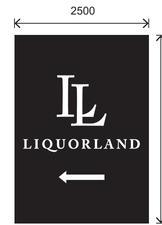
SIGN 5 WALL SIGN / NON - ILLUMINATED Flexface banner, digitally printed. QTY. 1 Size: 2500mmW x 3500mmH
