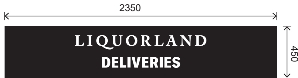
SIGN 2 DELIVERIES WALL SIGN QTY. 1 2mm Aluminium panel with digitally printed black with matt laminate. Size: 2350mmW x 450mmH
