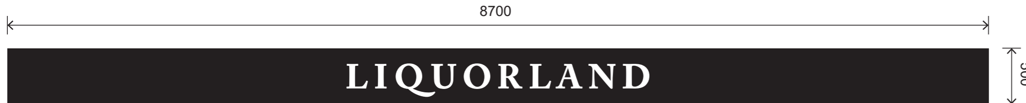
SIGN 3 CANOPY SIGN Non-illuminated QTY. 1 2mm Aluminium panel with digitally printed black with matt laminate, with all edges to be wrapped. Size: 8700mmW x 500mmH
