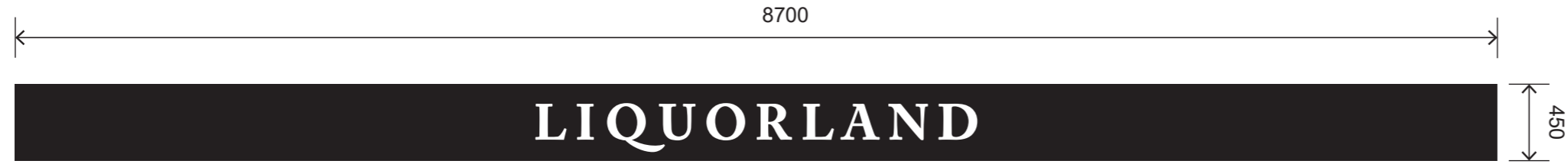
SIGN 1 FRONT CANOPY SIGN QTY. 1 2mm Aluminium panel with digitally printed black with matt laminate, with all edges to be wrapped. Size: 8700mmW x 450mmH
