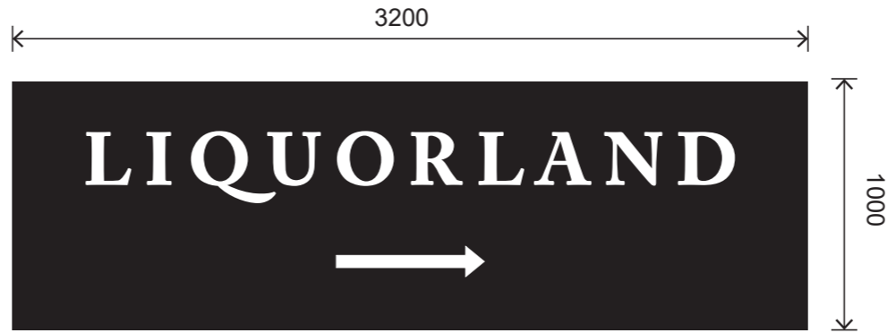
SIGN 5 DRIVE-THRU DIRECTIONAL SIGN QTY. 1 2mm Aluminium panel with digitally printed black with matt laminate, with all edges to be wrapped. Size: 3200mmW x 1000mmH
