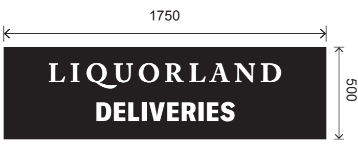
SIGN 4 DELIVERIES QTY. 1 2mm Aluminium panel with digitally printed black with matt laminate, with all edges to be wrapped. Size: 1750mmW x 500mmH
