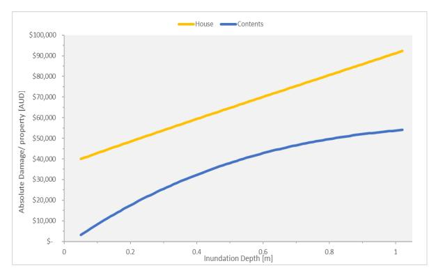
Figure 11 Residential Stage-Damage Curve (NRE, 2006)
