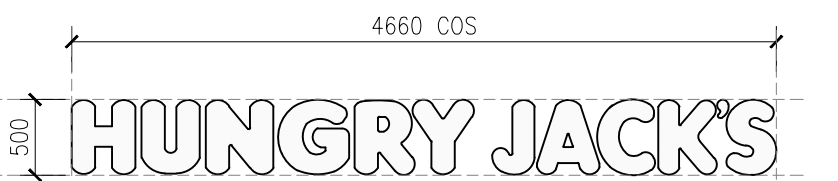
S16 ILLUMINATED LETTERSET DA06 SCALE 1:50 NEW INTERNALLY ILLUMINATED LETTERS WITH WHITE ACRYLLIC FACES. BLACK EDGES.
